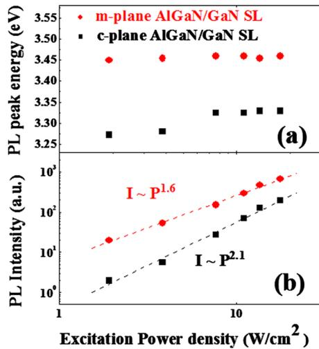
FIG. 3. (Color online) Dependence of (a) the PL peak position and (b) the PL peak intensity on laser excitation power density for  $\text{Al}_{0.2}\text{Ga}_{0.8}\text{N}(4.9 \text{ nm})/\text{GaN}(4.8 \text{ nm})$  SL grown on polar c- and nonpolar m-plane FS-GaN substrates.
