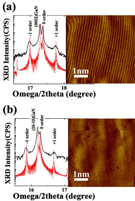
FIG. 1. (Color online) Omega/2theta XRD scan and simulation (left) and ( $5 \times 5 \mu\text{m}^2$ ) AFM image (right) of  $\text{Al}_{0.2}\text{Ga}_{0.8}\text{N}(4.9 \text{ nm})/\text{GaN}(6.4 \text{ nm})$  SL grown on (a) c-plane and (b) m-plane FS-GaN substrates.
