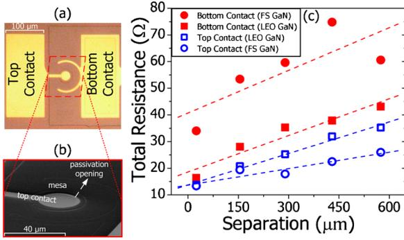
FIG. 1. (Color online) (a) Top-view optical micrograph of a fabricated RTD device, (b) SEM bird's eye view of a fabricated RTD mesa (zoomed-in), and (c) TLM measurements of top and bottom contacts of RTDs grown on LEO and FS GaN (each dashed line is the linear fitting to the respective TLM measurement).
