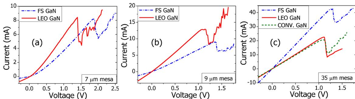
FIG. 2. (Color online) Electrical (I-V curve) measurements of RTDs grown on LEO GaN and FS GaN for various mesa diameters: (a) 7  $\mu\text{m}$ , (b) 9  $\mu\text{m}$ , and (c) 35  $\mu\text{m}$ . For comparison, I-V curve of (35  $\mu\text{m}$  in. diameter) RTD grown on CONV. GaN/sapphire is appended to Fig. 2(c).
