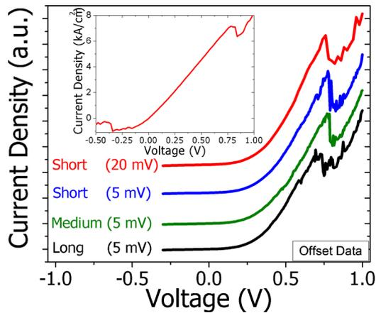
FIG. 3. (Color online) Electrical measurements (I-V curves) of RTDs under various measurement conditions [integration times of 640  $\mu$ s (short), 16.7 ms (medium), and 266 ms (long), and voltage sweep widths of 5 and 20 mV]. Inset shows the I-V curve of an RTD demonstrating NDR under both reverse and forward biases.
