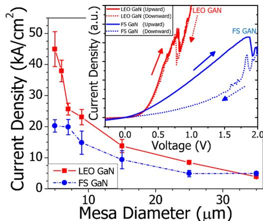
FIG. 4. (Color online) Dependence of  $J_{\text{NDR}}$  on the RTD mesa diameter. Inset shows the electrical hysteresis measurements of LEO and FS RTDs. The hysteresis curves are realized via measuring the device I-V from negative to positive voltage followed by positive to negative voltage—a loop of electrical I-V measurements.
