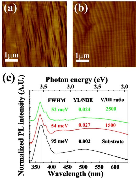
FIG. 1. (Color online) AFM image of 2  $\mu\text{m}$  homoepitaxial m-plane GaN grown at 1135  $^{\circ}\text{C}$ , and V/III=(a) 1500, and (b) 2500, (c) room temperature PL spectra of FS-GaN substrate and homoepitaxial m-plane GaN grown at V/III=1500 and 2500.
