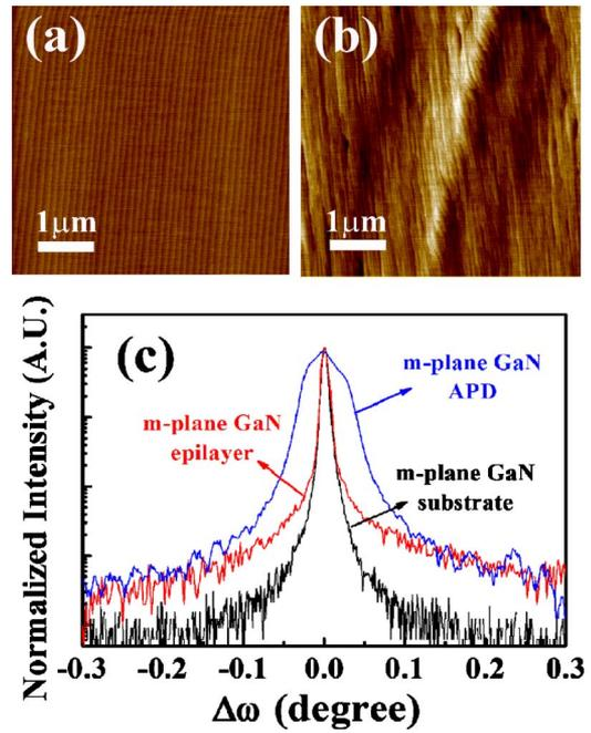
FIG. 2. (Color online) AFM image of (a) 2  $\mu\text{m}$  homoepitaxial m-plane GaN grown at 1150  $^{\circ}\text{C}$  and V/III=2500, and (b) m-plane GaN APD. (c) (10 $\bar{1}0$ ) XRCs of FS-GaN substrate, homoepitaxial GaN layer, and m-plane GaN APD.
