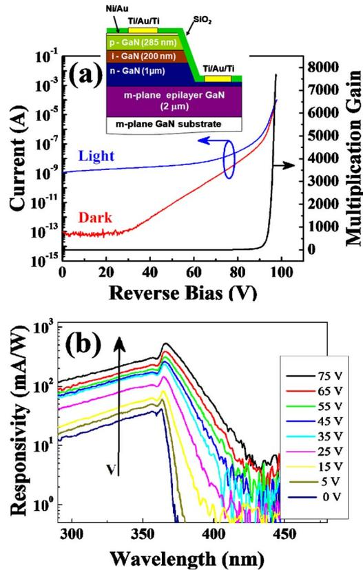
FIG. 3. (Color online) (a) I-V characteristics and gain of  $225 \mu\text{m}^2$  areas m-plane GaN APDs. Dark current and photocurrent are shown on the left axis; gain is shown on the right axis. The inset shows a cross-sectional diagram of the device structure. (b) Responsivity measurements with increasing reverse bias voltage (V).
