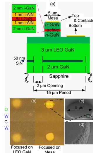
FIG. 3. (Color online) (a) The schematic view of the RTD, (b) the optical microscope image (focused on LEO GaN template and RTD mesa). The letters “O,” “W,” and “C” stands for opening, wing, and coalescence regions of the LEO GaN. (c) SEM image of an RTD mesa, and (d) SEM image of an RTD sidewall, top and bottom areas.
