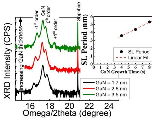
FIG. 2. (Color online) MOCVD growth calibration of the RTD active layer. X-ray diffraction of fifty periods of AlN/GaN SLs with different (1.7, 2.6, and 3.5 nm) GaN thicknesses (for a constant AlN thickness of 1.9 nm) are shown. The inset shows the SL period with respect to GaN growth time.
