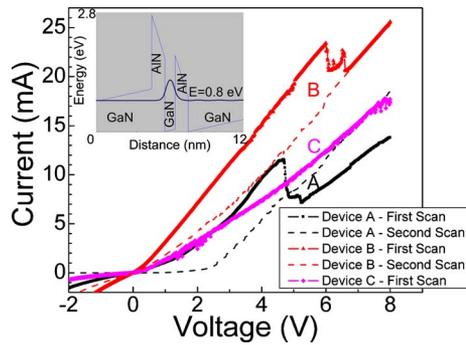
FIG. 4. (Color online) RT I-V curves, taken by sweeping voltage in positive direction while measuring current, of RTDs. Device A is on the wing where as from B to C mesa gets closer to opening (see Fig. 1). Inset displays the schematic conduction band diagram of DB active layer.
