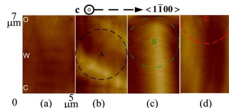
FIG. 1. (Color online)  $(5 \times 7 \mu\text{m}^2)$  AFM images of (a) EPD study of LEO GaN, (b) LEO GaN template, (c) RTD active layer, and (d) completed RTD structure. The letters “O,” “W,” and “C” stands for opening, wing, and coalescence regions of the LEO GaN. Circles A, B, and C denotes the relative location of RTD devices A, B, and C.
