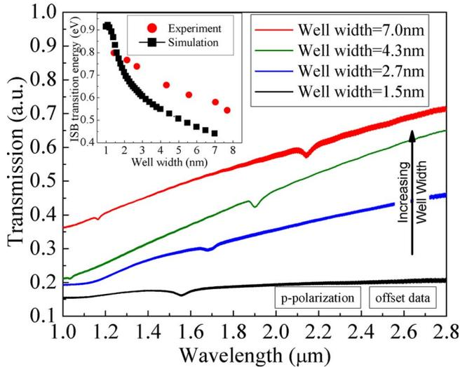
FIG. 4. (Color online) Transmission is plotted as a function of wavelength for four well widths of 1.5, 2.7, 4.3, and 7 nm. For all cases, AlN barrier thickness and growth temperature is 3.0 nm and 1035 °C, respectively. Inset shows simulated and observed ISB absorption energies as a function of well width (for the transition from the first state to the second state where other transitions are possible).
