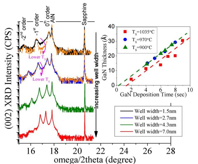
FIG. 3. (Color online) (002)  $\Omega/2\theta$  XRD of the SL with four well widths (all  $n$ -doped of  $1 \times 10^{18} \text{ cm}^{-3}$ ) of 1.5, 2.7, 4.3, and 7.0 nm, employing 3 nm thick barrier thickness, are plotted. All SL are grown at growth temperature ( $T_s$ ) of 1035 °C (solid). The XRD of 1.5 and 2.7 nm thick wells grown at 900 °C are also shown (dashed). Inset shows the GaN thickness as a function GaN deposition time for three different growth temperatures, 900, 970, and 1035 °C.
