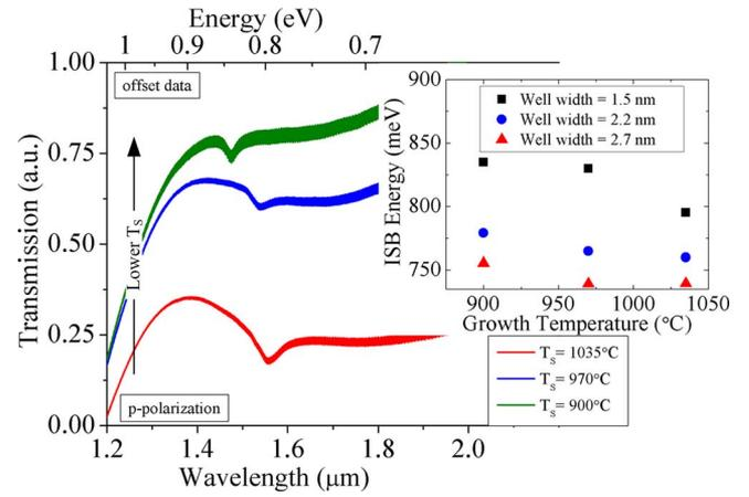
FIG. 2. (Color online) Transmission is plotted as a function of wavelength for three different growth temperatures, 900, 970, and 1035 °C for 50 periods of {1.5 nm thick GaN/3.0 nm thick AlN}. Wells are doped to  $1 \times 10^{18} \text{ cm}^{-3}$ . Inset shows ISB transition energy as a function of growth temperature for well widths of 1.5, 2.2, and 2.7 nm.
