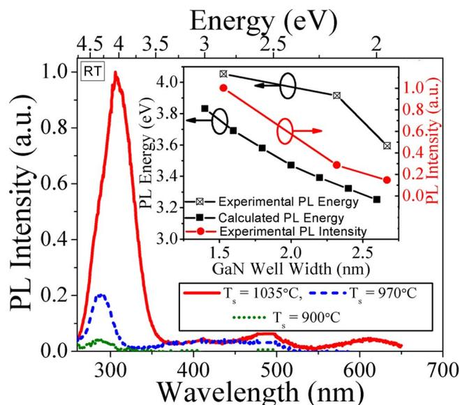
FIG. 1. (Color online) Room temperature PL intensity is plotted as a function of wavelength for three different growth temperatures, 900, 970, and 1035 °C for 50 periods of {1.5 nm thick GaN/3 nm thick AlN}. Wells are  $n$ -doped to  $1 \times 10^{18}$   $\text{cm}^{-3}$ . Inset shows the experimental (and simulated) PL energy as a function of well width [for the same barrier thickness and growth temperature ( $T_s$ ) of 1035 °C].
