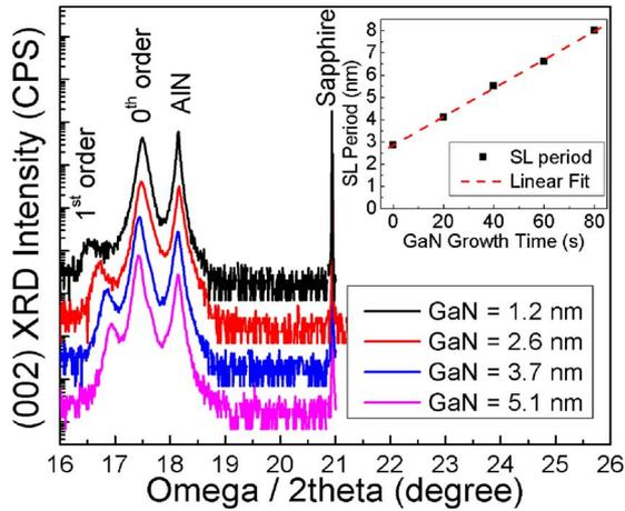
FIG. 1. (Color online) Omega/2theta (002) XRD of superlattices with four different well thicknesses: from top to bottom these are 1.2, 2.6, 3.7 nm and 5.1 nm GaN. Wells are Si doped to  $1 \times 10^{18} \text{ cm}^{-3}$ . The barriers for all samples are 2.9 nm thick  $\text{Al}_{0.2}\text{Ga}_{0.8}\text{N}$ . Inset: superlattice period (from XRD analysis) as a function of well growth time is used to extract the GaN growth rate and determine the well thicknesses.
