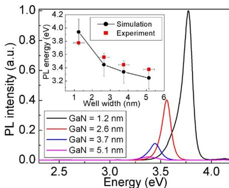
FIG. 2. (Color online) PL intensity as a function of energy for four different GaN well thicknesses: 1.2, 2.6, 3.7, and 5.1 nm—all with a constant 2.9 nm  $\text{Al}_{0.2}\text{Ga}_{0.8}\text{N}$  barrier thickness. Superlattice consists of 50 periods where each well is Si doped to  $1 \times 10^{18} \text{ cm}^{-3}$ . Inset: Comparison theory/experiment PL energy as a function of well width.
