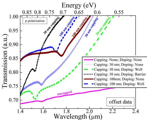
FIG. 4. (Color online) Relative (*p*-polarization) transmission of undoped, well- or barrier-doped, and uncapped, 30 or 100 nm capped 50 period {1.9-nm-thick GaN/3.2-nm-thick AlN} SL.
