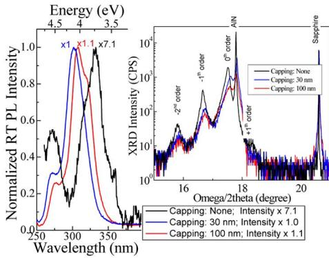
FIG. 3. (Color online) Room temperature PL of 50 periods {1.9-nm-thick GaN/3.2-nm-thick AlN} SL with different AlN capping thicknesses (uncapped, 30, and 100 nm). Inset shows (002) omega/2theta XRD of the SL with the different capping thicknesses.
