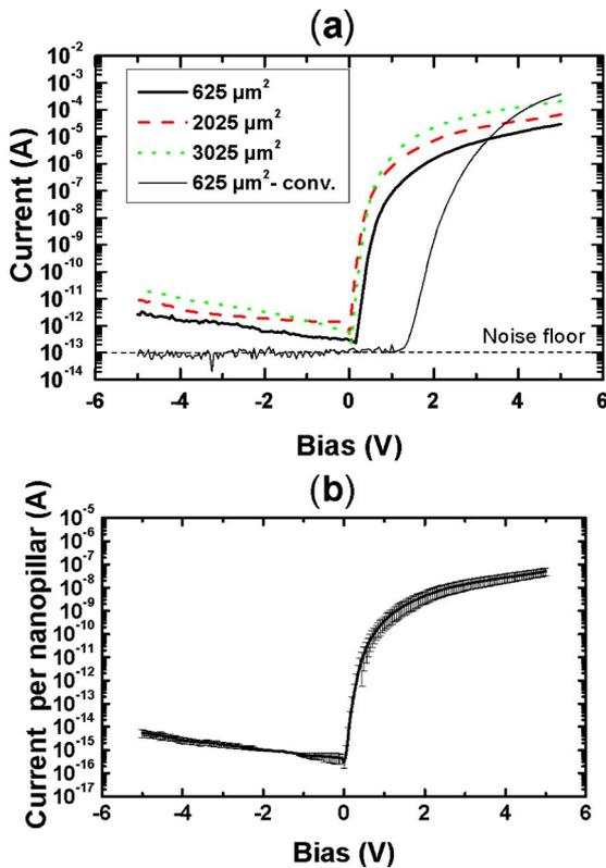
FIG. 2. (Color online) (a) Current-voltage characteristics of GaN nanostructured  $p$ - $i$ - $n$  diodes with different device areas ( $625$ ,  $2025$ , and  $3025 \mu\text{m}^2$ ) as compared to  $625 \mu\text{m}^2$  conventional diodes. (b) Average current-voltage characteristic per nanopillar and error bars (standard deviation) obtained from the measurement of 30 diodes.
