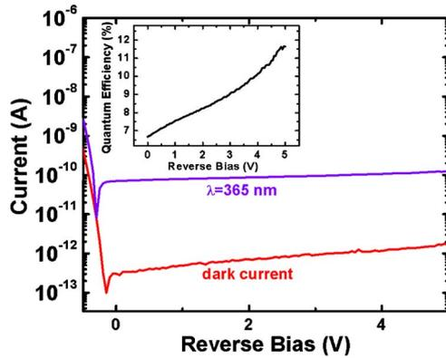
FIG. 4. (Color online) Reverse current of a  $625 \mu\text{m}^2$  diode in darkness and under back-side illumination at 365 nm. Inset: calculated QE as a function of bias.
