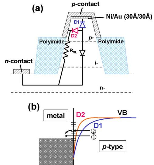
FIG. 3. (Color online) (a) Nanopillar cross section and schematics of the proposed model. (b) Valence band bending at the top (D1) surface of the nanopillar and sidewalls (D2) in the  $p$ -GaN region and proposed tunneling mechanisms.
