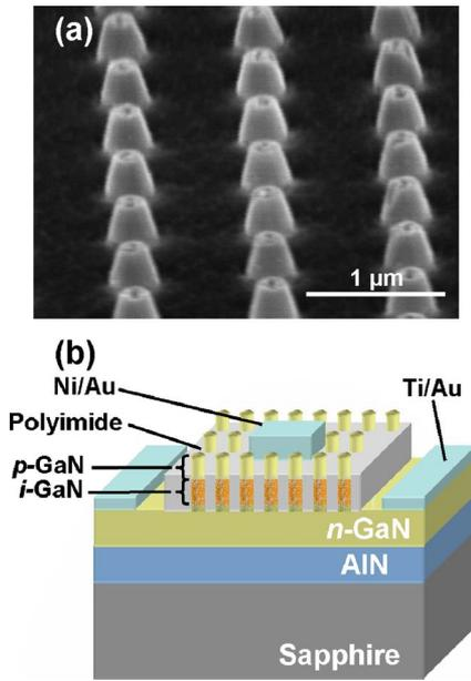
FIG. 1. (Color online) (a) SEM image of the nanopillar array after polyimide deposition and etch back. (b) Schematic of the device.
