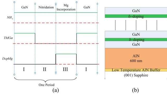
FIG. 2. (Color online) (a)  $\delta$ -doping profile implementation. (b) Side view of the  $\delta$ -doped  $p$ -GaN structure.
