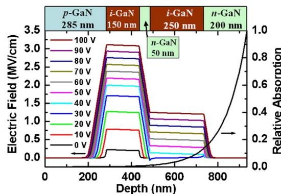
FIG. 1. (Color online) Left axis: electric field profile calculated as a function of reverse bias in the SAM APDs. Right axis: relative absorption for an absorption coefficient of  $1 \times 10^5 \text{ cm}^{-1}$ . The basic structure of the device is depicted at the top.
