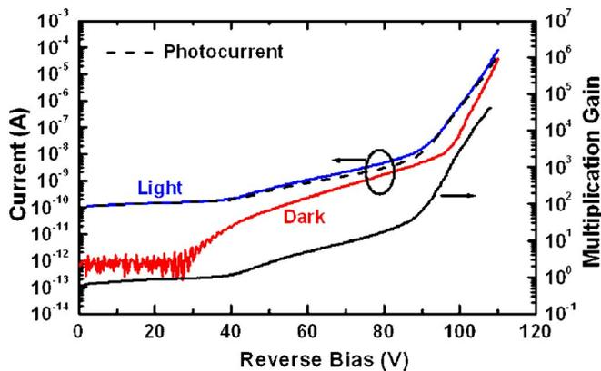
FIG. 2. (Color online) Left axis: dark and light (360 nm) currents measured in the SAM APDs; the dashed line represents the calculated photocurrent. Right axis: calculated gain.
