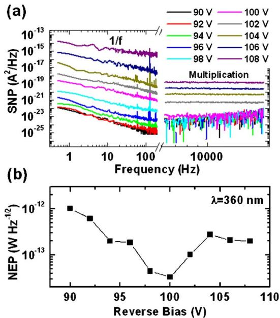
FIG. 4. (Color online) (a) Spectral noise power obtained near breakdown. The broken  $x$  axis separates the low frequency range, in which the  $1/f$  contribution dominates, from the midfrequency range, dominated by the multiplication noise. (b) Calculated NEP vs reverse bias voltage.
