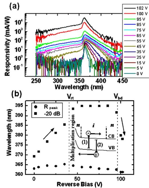
FIG. 3. (Color online) (a) Spectral response measured in the SAM APDs as a function of reverse bias. (b) Wavelength of the responsivity peak ( $R_{peak}$ ) and 20 dB fall-off wavelength ( $-20$  dB) as a function of reverse bias. The arrows indicate the redshift of the response cutoff at low voltages and the blueshift induced by the multiplication process near breakdown. The inset shows the band tailing absorption processes that may account for this behavior.
