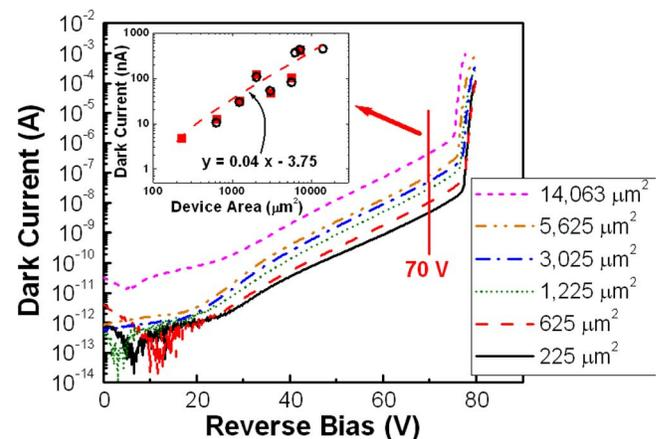
FIG. 1. (Color online) *I-V* curves for circular mesa devices of increasing area. The inset plots the dark current value at 70 V reverse bias for both square (red squares) and circular (open circles) mesas with increasing area.
