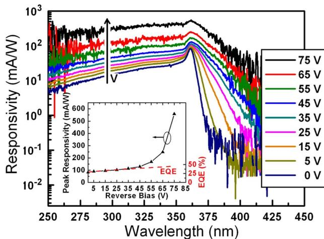
FIG. 2. (Color online) Responsivity measurements with increasing reverse bias. The inset plots the peak responsivity with increasing bias and the extracted external quantum efficiency fit.
