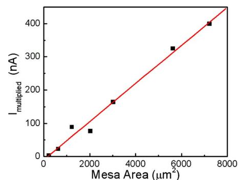
FIG. 4. (Color online) Multiplied current component of the dark current as a function of mesa area.
