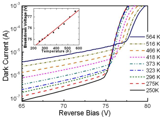
FIG. 5. (Color online) Temperature-dependent evolution of the breakdown from 250 to 564 K for a  $14\,063\ \mu\text{m}^2$  device. The inset plots temperature vs breakdown voltage demonstrating a positive thermal coefficient of  $+8.3\ \text{mV/K}$ .
