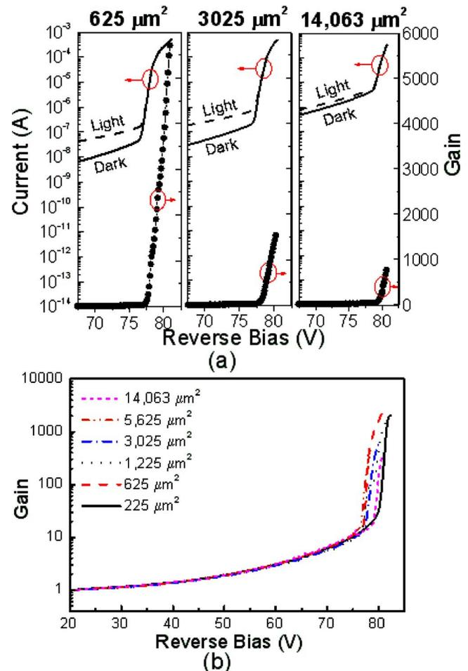
FIG. 3. (Color online) (a) Light current, dark current, and gain curves around breakdown from 625, 3025, and 14 063  $\mu\text{m}^2$  avalanche photodiodes. (b) Gain vs reverse bias for several mesa areas.
